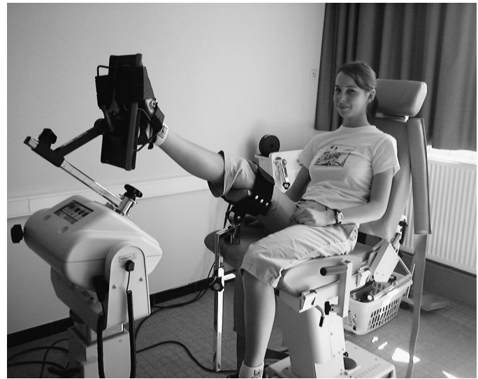
Figure 2. Positioning of the subject for testing isokinetic ankle inversion/eversion on the Biodex 3 isokinetic dynamometer.
